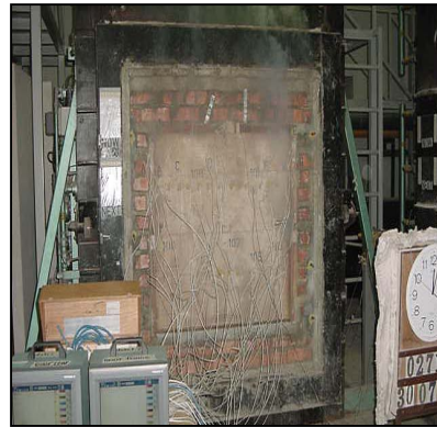
Figure 1: Scaled furnace testing – “Cube Test”.
