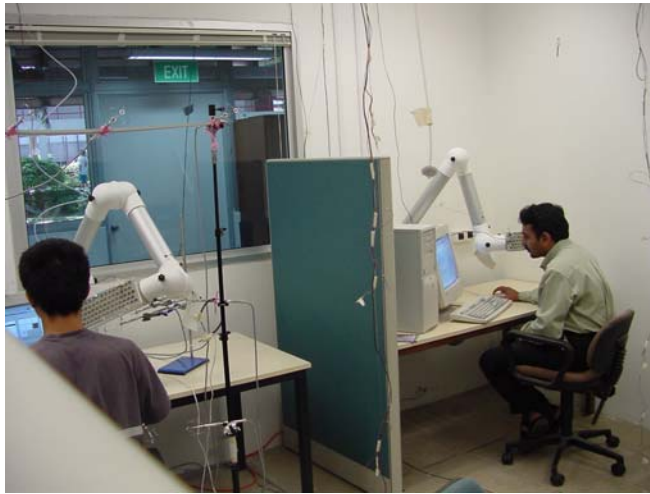
Figure 4. Personalised Ventilation (PV) experiments in the IAQ Chamber.
