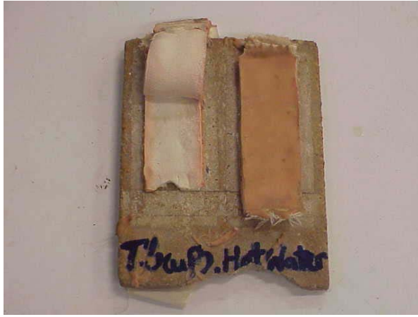
Figure 3. 100% cohesive failure was shown in the peel-adhesion test (ASTM C794) of this sealant to concrete without primer after a 28-day immersion in 70°C water. (The larger the percentage of cohesive failure given by ASTM C794, the stronger the peel adhesion.)
